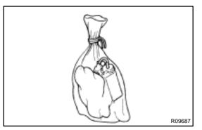
3. DEPLOYMENT WHEN DISPOSING OF FRONT PAS-SENGER AIRBAG ASSEMBLY WITH AIRBAG DEPLOYED IN COLLISION
